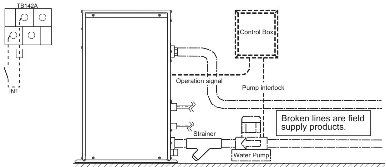
Example drawing for pump interlock
