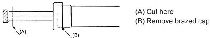
2. Pull out the thermal insulation on the site refrigerant piping, braze the unit piping, and replace the insulation in its original position.
