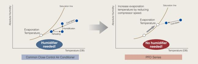
This system will also help to minimize maintenance costs by removing the need for a humidifier and doing away with the need to install water pipes for individual units.
