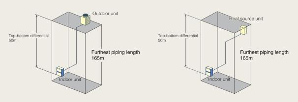
$\ensuremath{\mbox{\sc \#}}$  Same length with two refrigerant circuit connection
