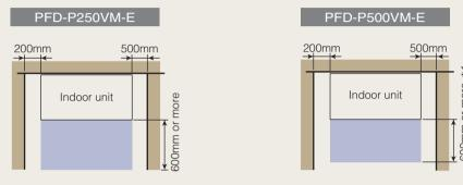
\*1. To open the gate fold maintenance pannel fully, space of 1000mm or more required.
