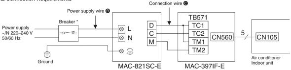
\* Connect the power switch with gap of 3 mm or more when open to interrupt the source power phase. (When the power switch is shut off, it must interrupt all phases.)
