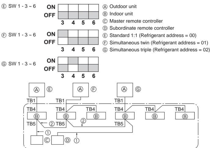
\* Set the refrigerant address using the DIP switch of the outdoor unit.
