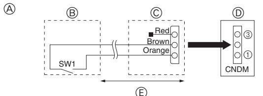
(A) Circuit diagram example (low noise mode)
