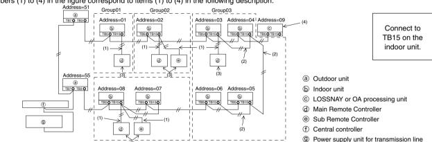
• Connect to the MA remote controller terminal block (TB15) on the indoor unit.
