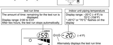
and indoor unit piping temperature. Make this setting only when interlocked operation with LOSSNAY or OA processing unit is 6 | Ventilation Setting necessary with CITY MULTI models.
