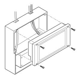
If the LAN link-up cable is used, place it inside the Mounting attachment A type as shown in the figure below.
