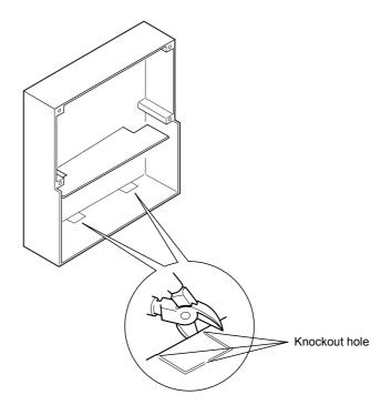
(3) Sand the cut surface of the knockout hole smooth.
