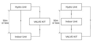
VALVE KIT Indoor Unit Auto air vent valve (Highest point on the water pipe)(field supply) VALVE KIT Indoor Unit or less Air vent valve (field supply) is needed to highest point.
