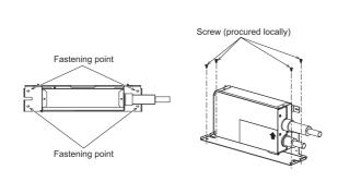
Installation pattern C (vertical surface installation method)
