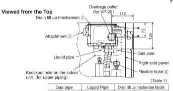
Installing the Drain lift up mechanism
