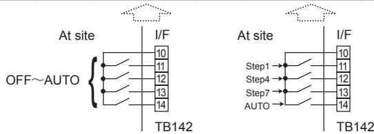
Demand control is available by connecting remote switches with terminal No.10 - 14.
