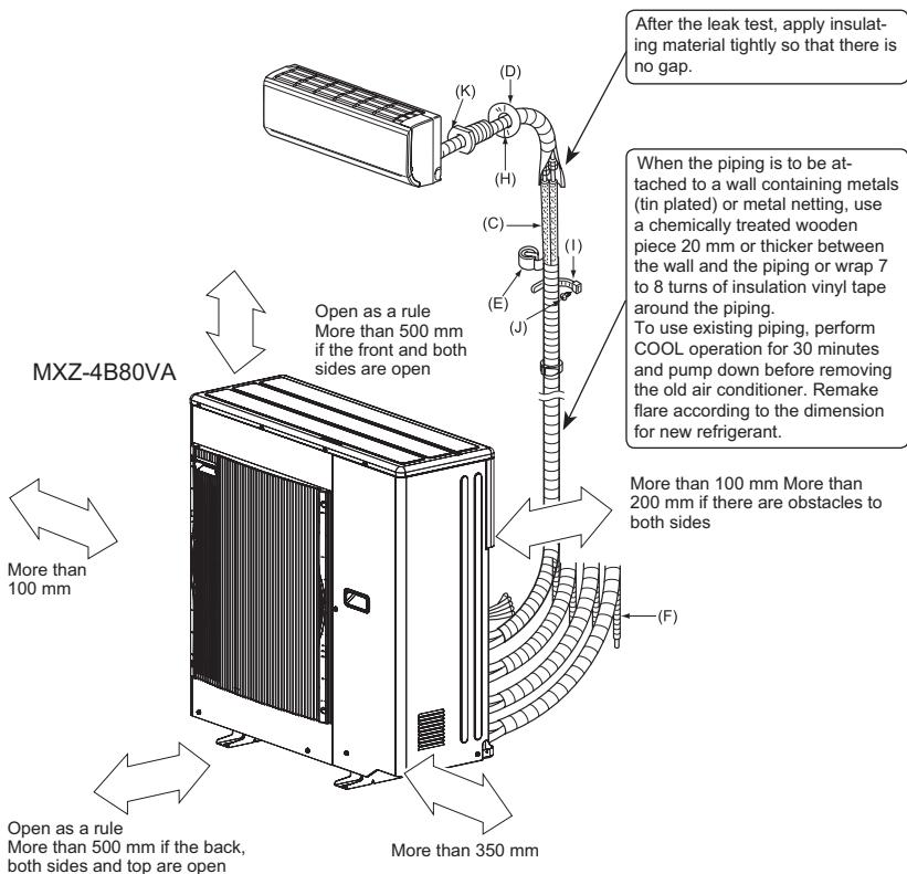
Units should be installed by licensed contractor according to local code requirements.
