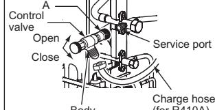
When attaching the control valve to the service port, valve core may deform or loosen if excess pressure is applied. This may cause gas leak.
