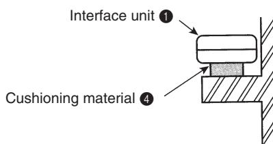
When mounting the interface unit ① inside a ceiling or wall, install an access door to facilitate maintenance.
