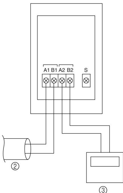
**When the connecting wires A are cross-wired**
