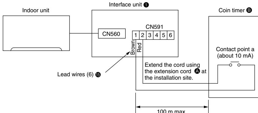
\* When the contact point is open, the unit will turn off and will not be operable from the remote control.
