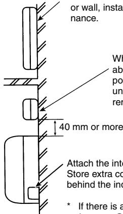
When the interface unit ① is mounted above an indoor unit, it should be positioned 40 mm or more away from the unit to ensure that ceiling grills can be removed.
