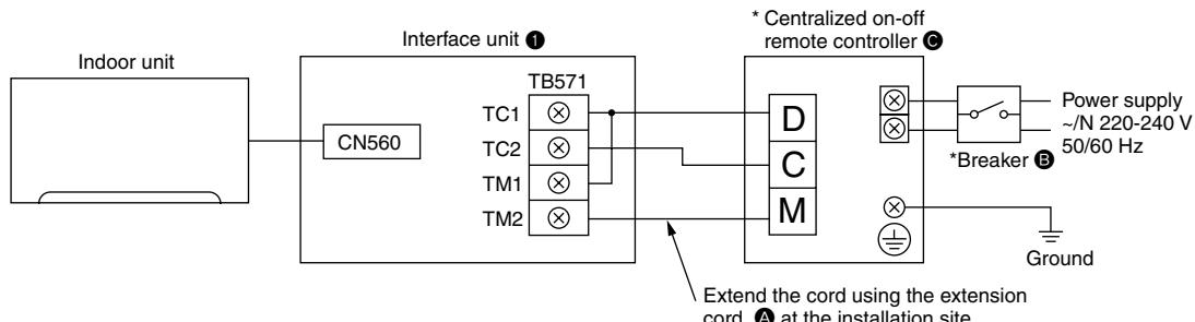
\* Refer to the installation manual of centralized on-off remote controller.
