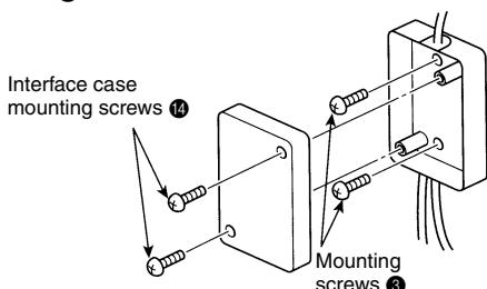
\* When mounting the interface unit ① using a cushioning material ④, be sure to mount it in a location where it will not fall.
