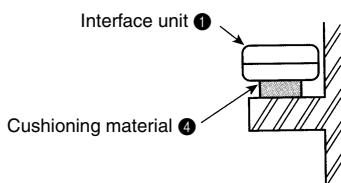
When mounting the interface unit ① inside a ceiling or wall, install an access door to facilitate maintenance.
