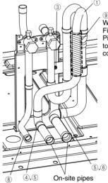
Wrap the pipe cover here. Fix compressor cables to Pipe cover with Cable tie to keep them out of direct contact with the pipes.
