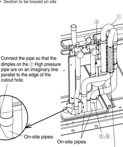
Wrap the pipe cover here. Fix compressor cables to Pipe cover with Cable tie to keep them out of direct contact with the pipes.
