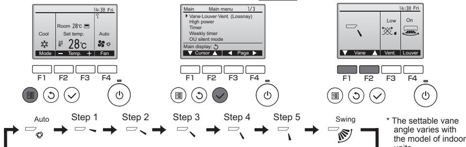
\* The settable vane angle varies with the model of indoor units.
