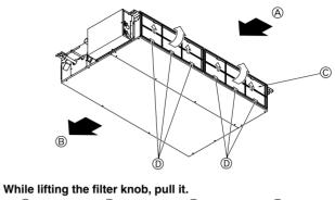
Air intake B Air outlet C Filter D Knob
