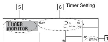
1. Be sure that the simple timer indicator is visible on the screen (at ①).
