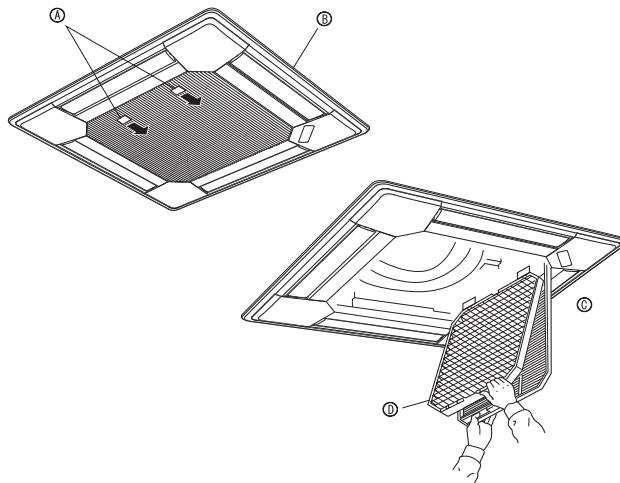
① Pull the knob on the intake grille in the direction indicated by the arrow and it should open.
