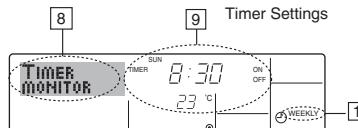
1. Be sure that the weekly timer indicator is visible on the screen (at [1]).
