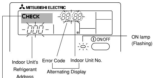
If you have entered contact number to be called in the event of a problem, the screen displays this number. (You can set this up under Function Selection of remote controller. For information, refer to Installation Manual.)
