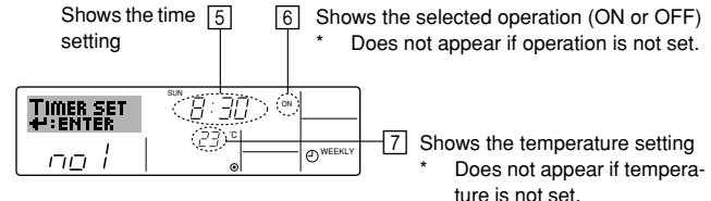
5. Press the appropriate Set Time button ⑪ as necessary to set the desired time (at ⑤).
