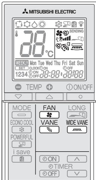
Press **FAN** to select fan speed. Each press changes fan speed in the following order:
