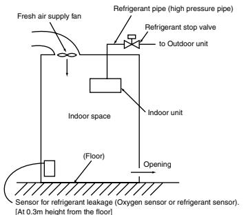
Fig.6-(2)-D. Fresh air supply and refrigerant shut-off upon sensor action
