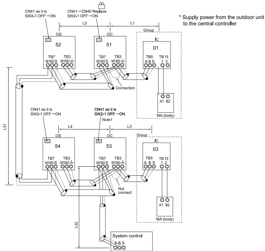
Note 1. When only the LM adapter is connected, leave SW2-1 to OFF (as it is).
