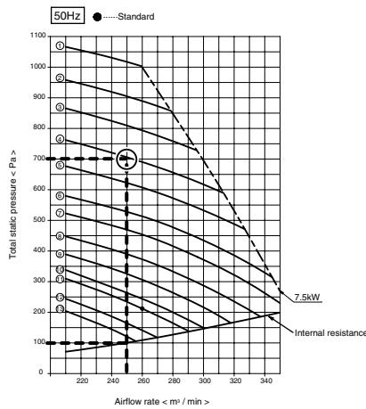
The fan characteristic curve shows the internal resistance is 100 Pa when the air flow rate is 250m<sup>3</sup>/min.
