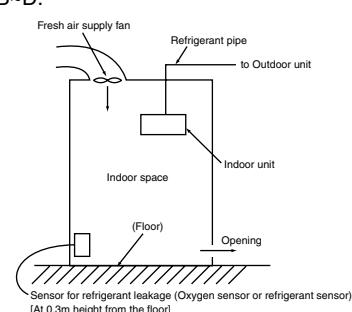
Fig.6-(2)-C. Fresh air supply upon sensor action
