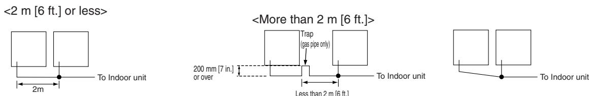
When installing the twinning kit in a higher position than the outdoor unit base, make sure that the twinning kit is installed in a position lower than 200 mm [7 in.] from the outdoor unit base.
