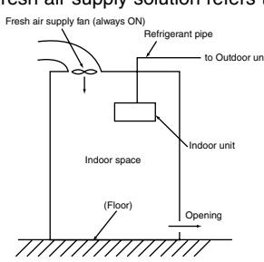
Fig.6-(2)-B. Fresh air supply always ON
