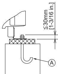
Install the unit in such a way that the corner of the angle bracket at the base of the unit shown in the figure is securely supported. The brackets may bend if they are not securely supported.
