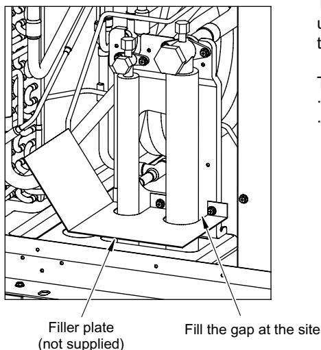
The gaps around the edges of through holes for pipes and wires on the unit allow water or mice to enter the unit and damage its parts. Close these gaps with filler plates.
