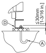
Install the unit in such a way that the corner of the angle bracket at the base of the unit shown in the figure is securely supported. The brackets may bend if they are not securely supported.
