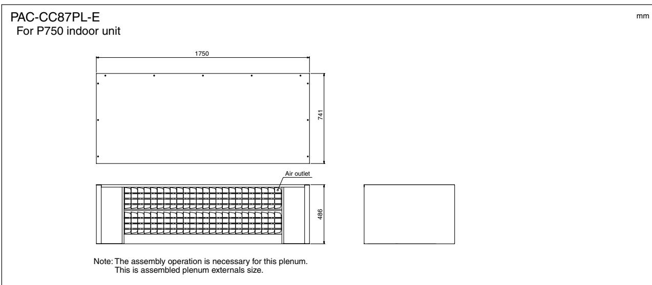
Note 1. The external static pressure in the plenum chamber is 30 Pa.
