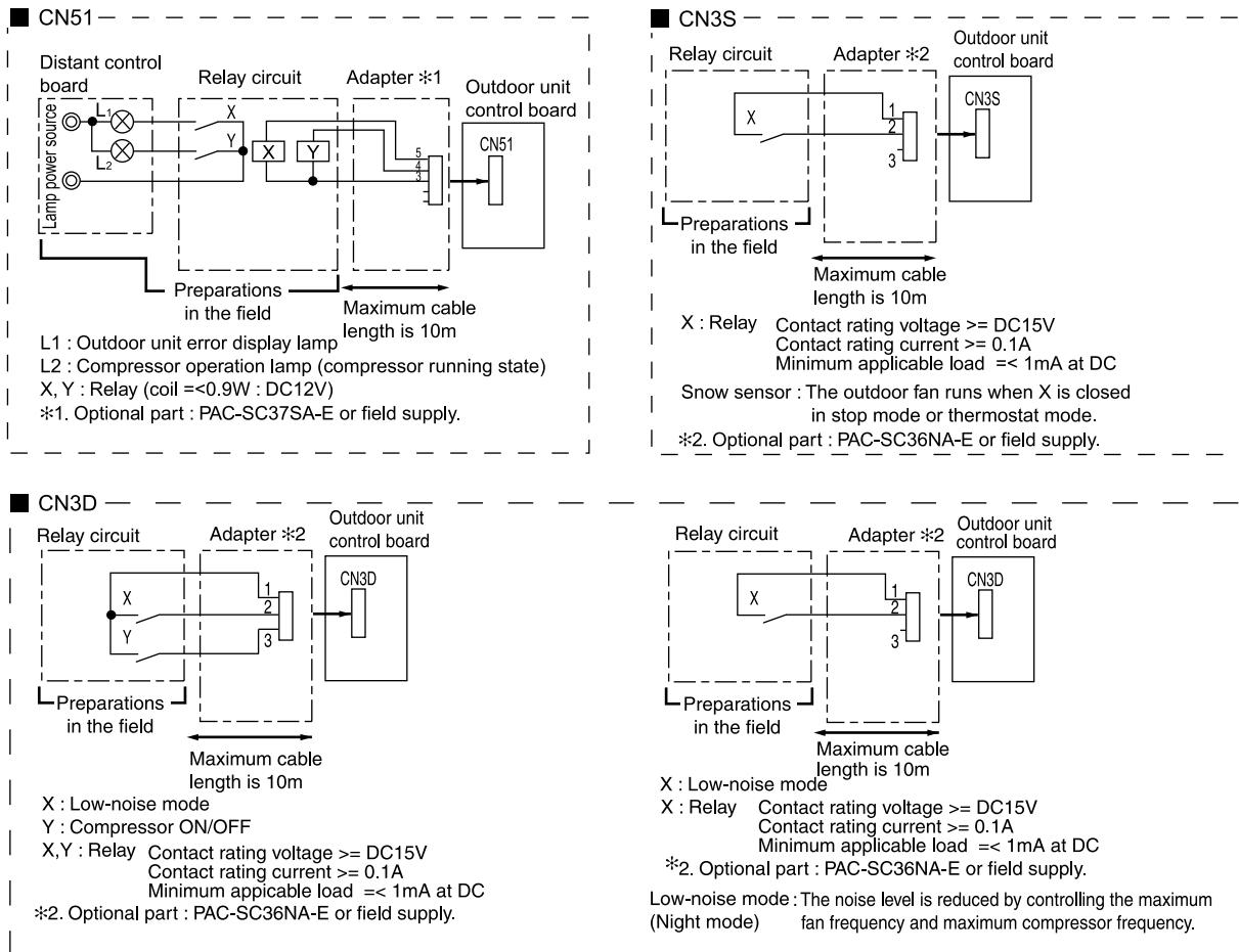
1) SW4-4: OFF (Compressor ON/OFF, Low-noise mode)
